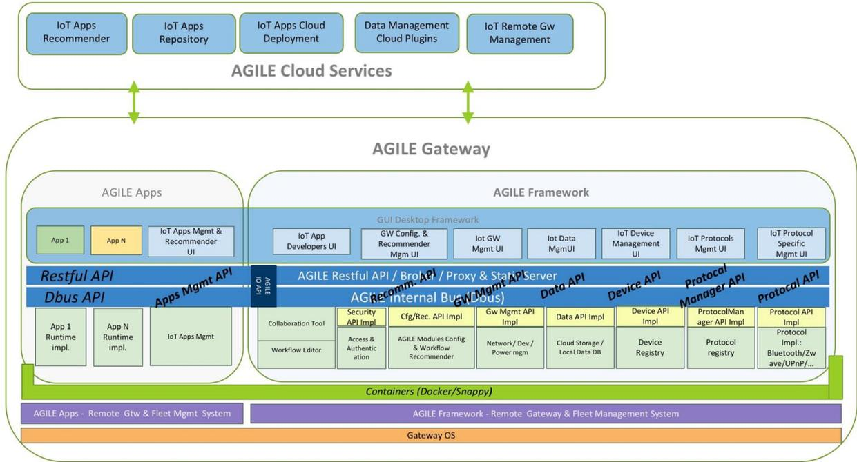
Figure 2: The AGILE Microservices Architecture
