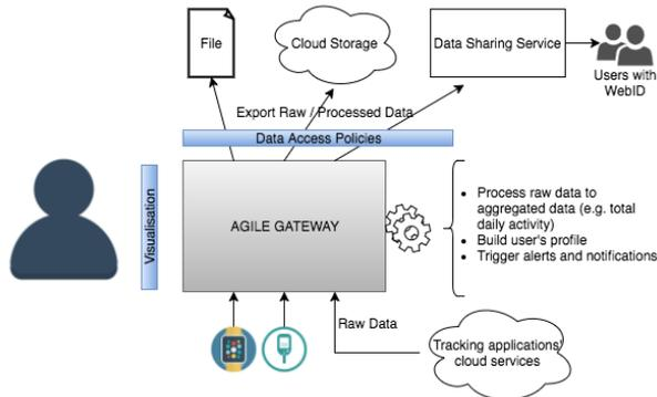
Figure 4: Quantified-Self Data Flow Overview
